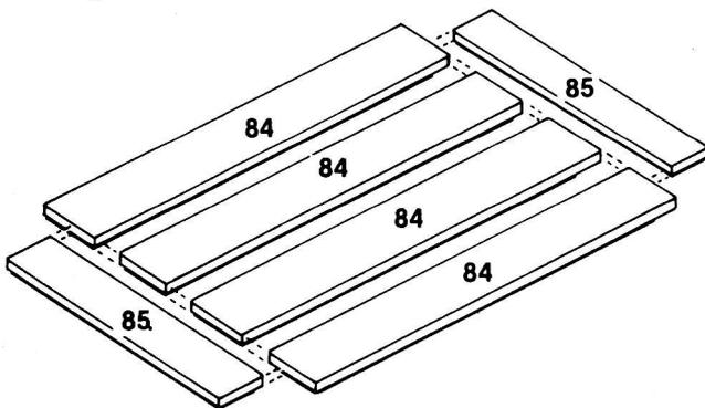
A. Glue the four top pieces (84) together. Care should be taken to align ends and top surfaces. Allow glue to set.
