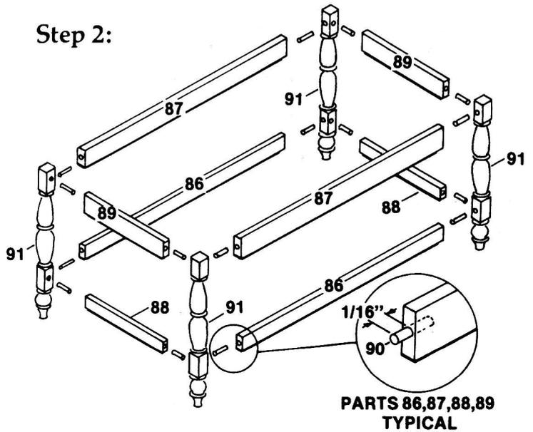
A. Sand all parts. Use the dowel (90) provided and glue pegs into ends of spreaders (88 & 86) and top rails (87 & 89). Dowel should project 1/16" (See inset)
